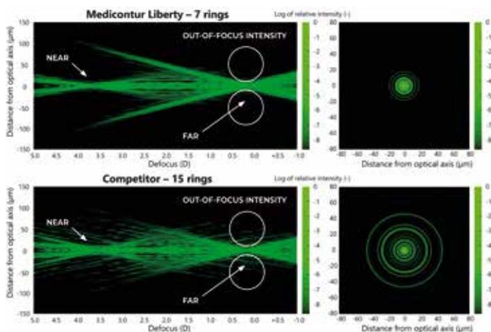
Fig. 8: Light Energy Intensity at 4.5 mm Aperture simulated by Zemax for calculation of light propagation after custom defining diffractive surfaces shows less out-of-focus light with the Liberty trifocal compared to a diffractive profile with 15 diffractive rings
